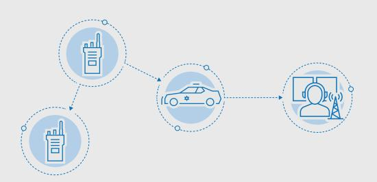
VRX1000-equipped vehicle extends simplex communications from portable radios to dispatch
