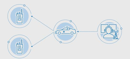
VRX1000-equipped vehicle extends simplex communications to portable radios from dispatch
